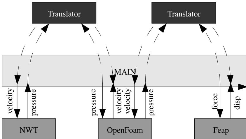
Figure 2: Software implementation and data exchange between components
